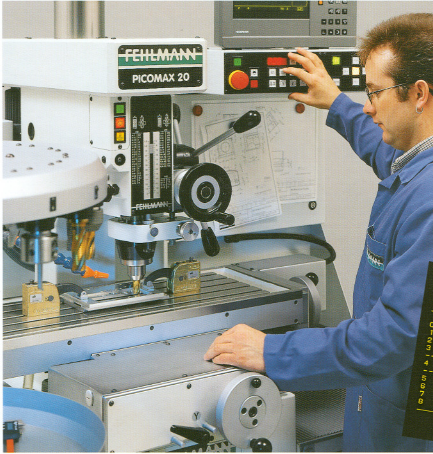
Hole circle machining with operator prompting.
